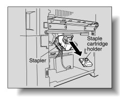
**3** Remove the empty staple cartridge from the staple cartridge holder.
